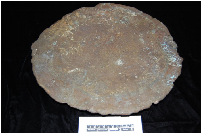
Figure 1 Upper surface of a copper Reißscheiben ingot from a 16th century wreck off the Kent coast.
