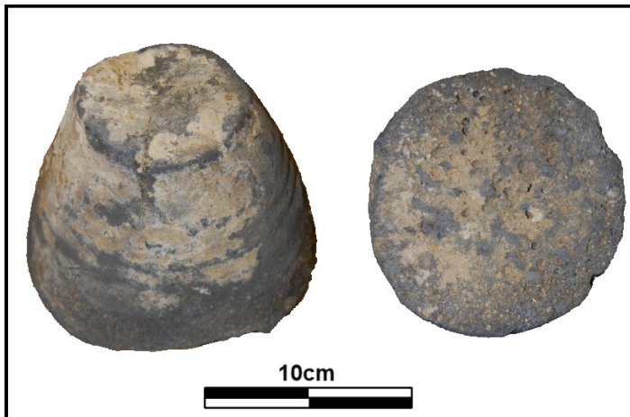
Figure 5 Ingot of stibnite (shown inverted-Left) from a 17th century wreck off the Kent coast. The molten stibnite would have dripped down into a crucible whose form is preserved here. Right-Upper surface with preserving gas bubbles generated as the mineral cooled and set.
