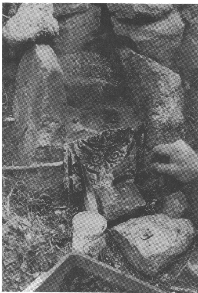
Figure 10. Blowing furnace at work. The molten tin metal can be seen flowing along the groove in the float stone. Slag and charcoal are being pushed aside with a spoon. The light glow from the "eye" is mainly blue producer gas flame.
