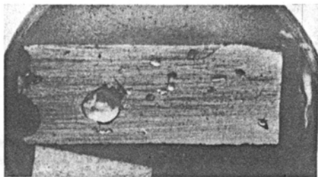
Fig. 2 — Section A-B, showing the large casting voids through which the sword was fractured × 3
