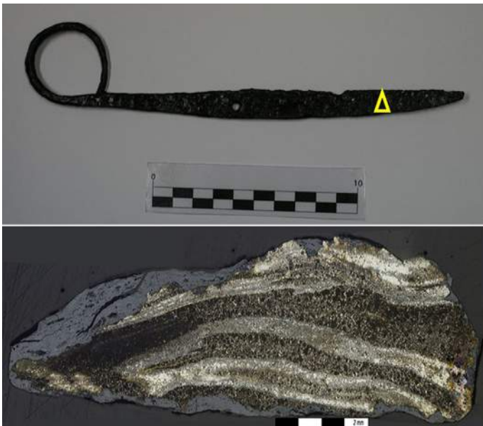
Fig. 3 Scissors found in Zaballa dating 8th to 10th century AD and micrograph showing the complex banded structure alternating phosphoric iron and martensite.
