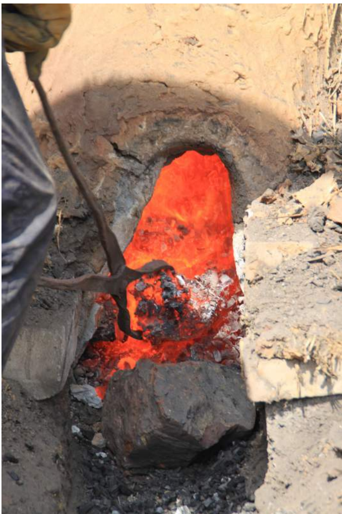
Removing the solidified slag mass from furnace 1.
