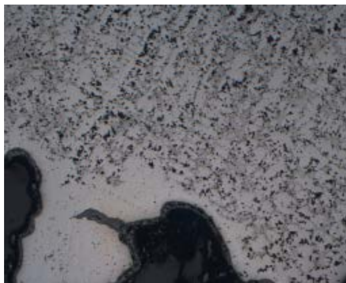
Fig. 1. Metallographic section showing the dendrites of ferritic iron with slag around the edges
