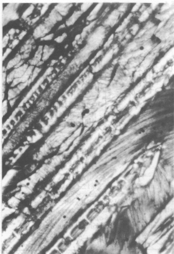
(a) Skeletal olivine, showing inclusions of matrix material within crystals; and obscurely crystalline matrix.
