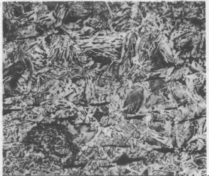
Figure 2a Microstructure of 'currency bar', showing the Widmanstatten distribution of ferrite, and slag particles. x 74. (B. Gilmour).
