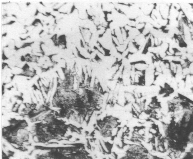
Figure 8 Saxon spearhead. Transverse section from rear socket, showing transition from low carbon area to carburised region on outside. Ferrite (white), and coarse lamellar pearlite (dark). x 375
