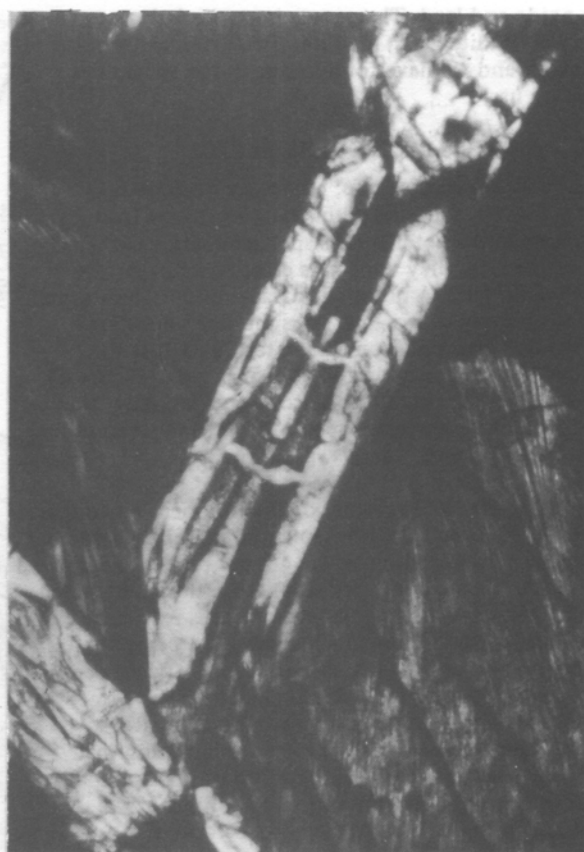
(b) Single skeletal olivine crystal. The upper left field is dark, indicating non-crystallization of the matrix. Incipient crystallization is shown lower right.
