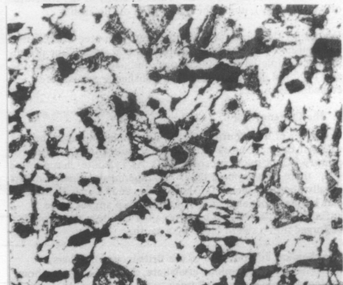
Figure 3 'Currency bar'. Region of intermediate carbon content, showing grains of ferrite (white) and lamellar pearlite (dark), and some slag. x 400 (B. Gilmour)
