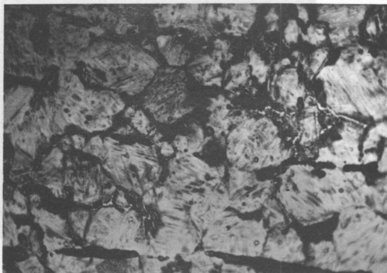
Section 1. Martensite (light grey), pearlite (dark) and grain-boundary ferrite (white). Etching: Picral 400 x.
