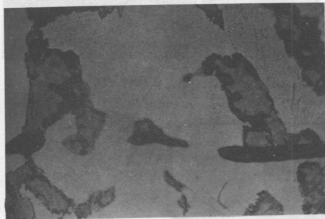
Section 2. Matrix with ferrite and grains of both martensite and pearlite, Etching: Nital: 950 x.
