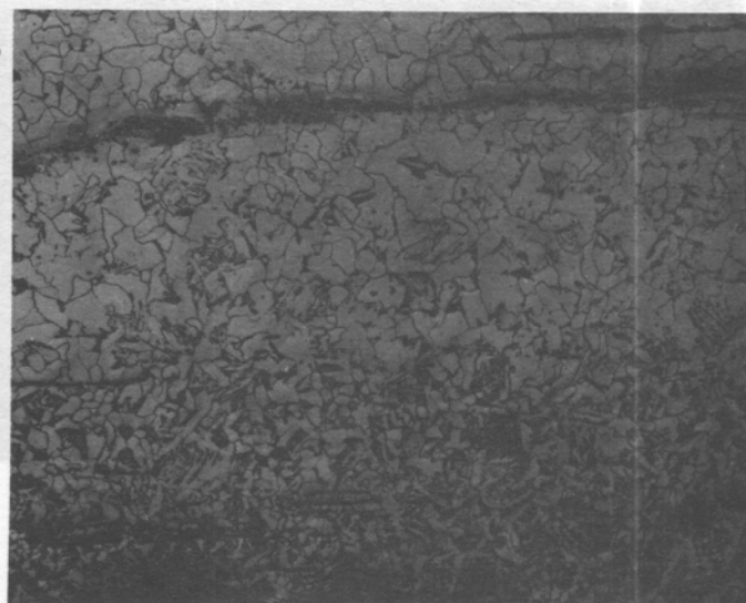
Section 8. Area of ferrite and pearlite. At the top a diffuse, martensitic streak is seen. Etching: Nital. 60 x.
