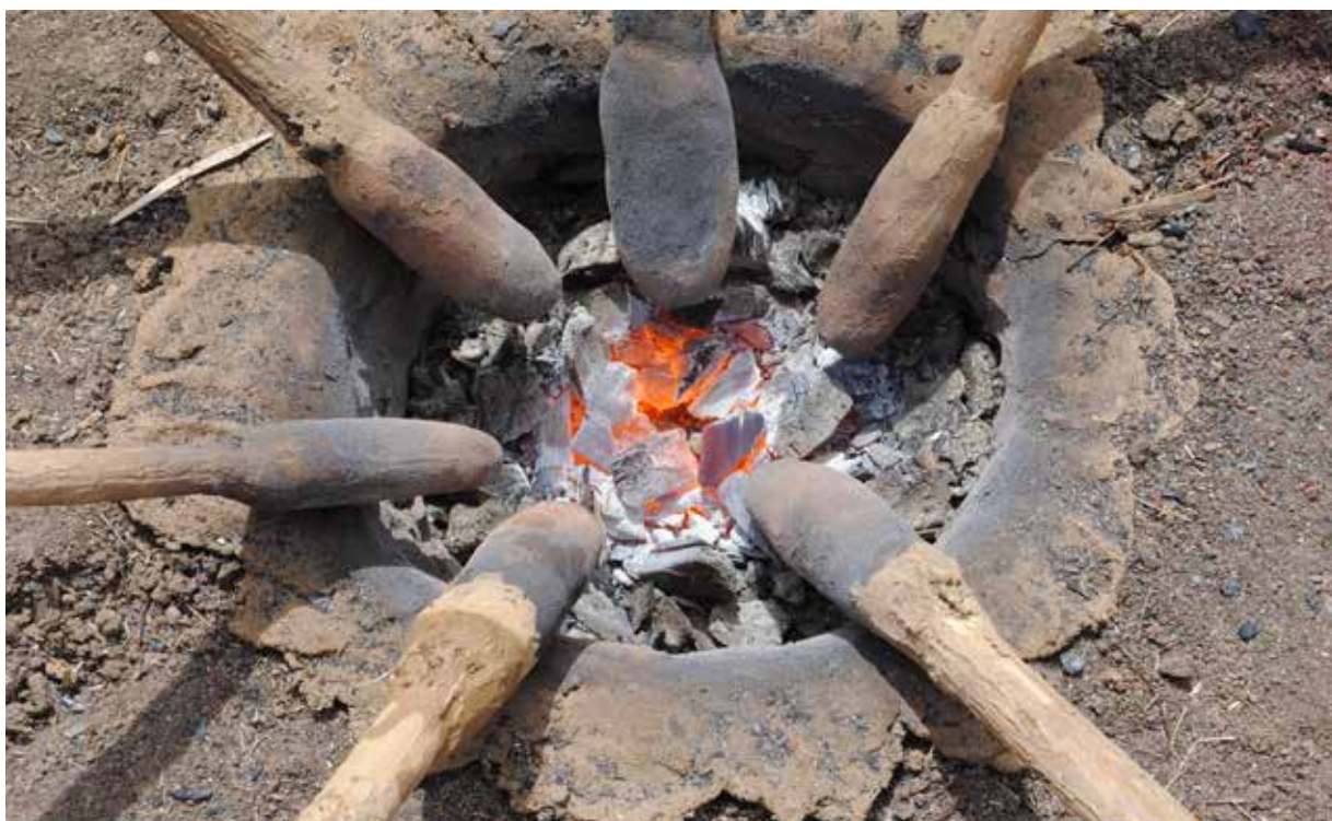
Copper smelting in Serbia using ceramic tipped blow pipes.
