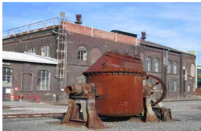
Bessemer located at the Henrichshütte Bessemer works in Hattingen, Germany. It belonged to the Eisenwerke Rödinghausen company.
