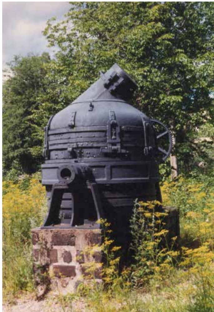
The Västanfors bruk Bessemer converter currently in Fagwersta, Sweden.
