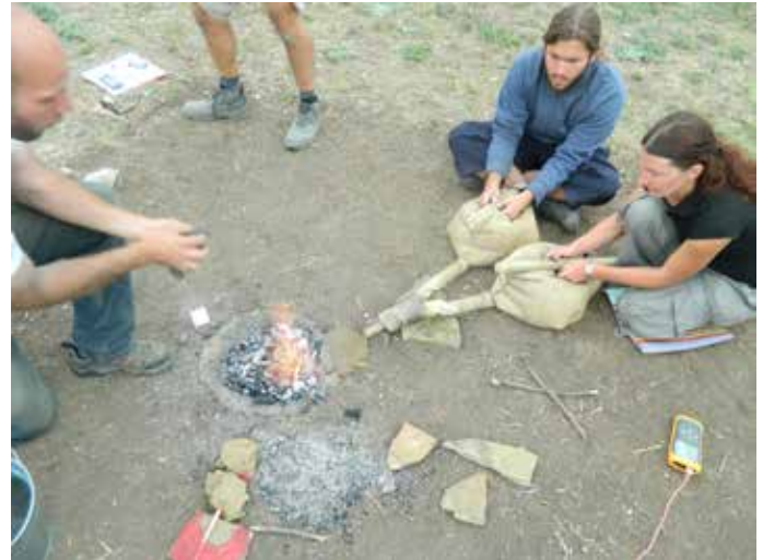
Charging the bellows-powered smelting installation with hornbeam charcoal.
