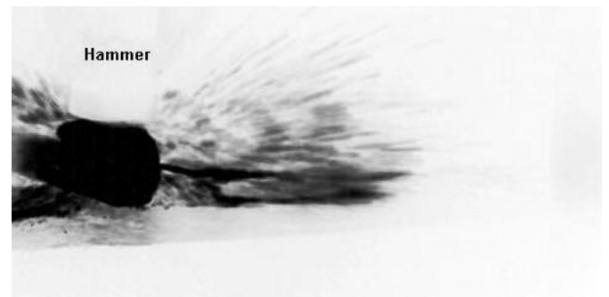
Figure 3. Still from high-speed digital film of welding. 0.007 seconds after the hammer struck the iron (negative image)
