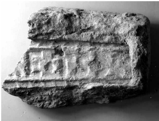
Figure 1. Skillet handle mould fragment (reversed image to show the inscription as it would appear on the casting)
