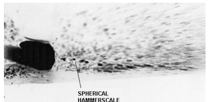
Figure 5. Still from high-speed digital film 0.017 seconds after the hammer struck (negative image)
