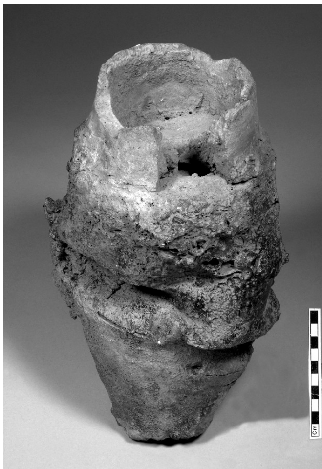
Figure 1. Zinc-smelting retort from Yangliusi, British Museum Reg. 2008, 3006.1. (BM / T. Springett)
