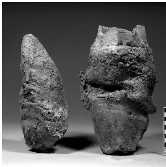
Figure 2. Zinc-smelting retorts from India and China, almost certainly the first time that such retorts have ever been together. Although contemporary the processes are totally different; in the Indian process the zinc vapour descends, in the Chinese process it rises. (BM / T. Springett)
