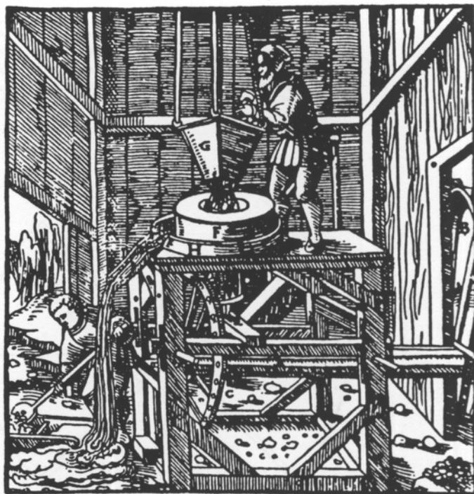
A—AXLE. B—WATER-WHEEL. C—TOOTHED DRUM. D—DRUM MADE OF BUNDLES. E—IRON AXLE. F—MILLSTONE. G—HOPPER. H—ROUND WOODEN PLATE. I—TROUGH.
