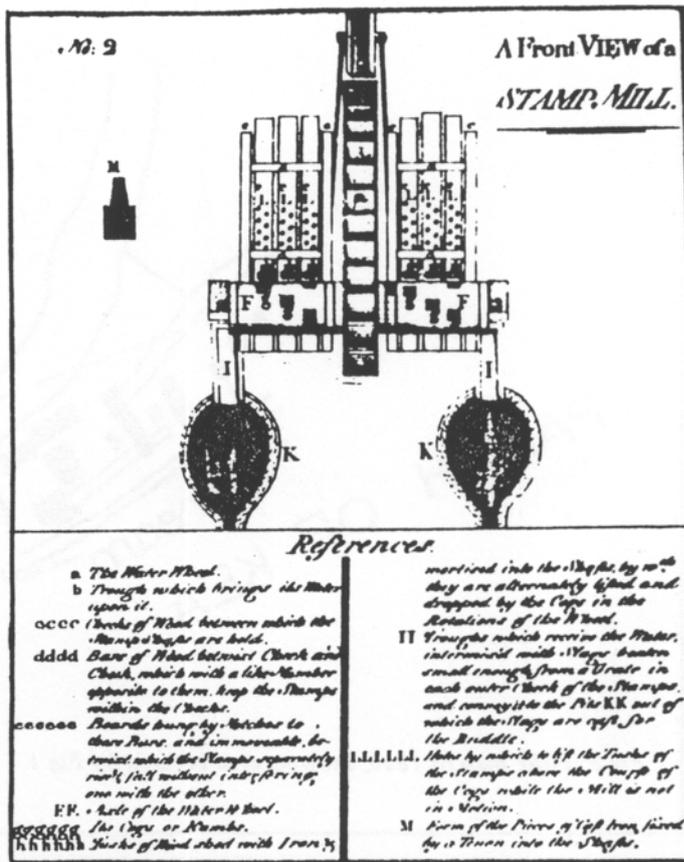
Fig 7 Stamps used for lead ore in the Northern Pennines and said to be based on those used in Cornwall (Mulcaster).
