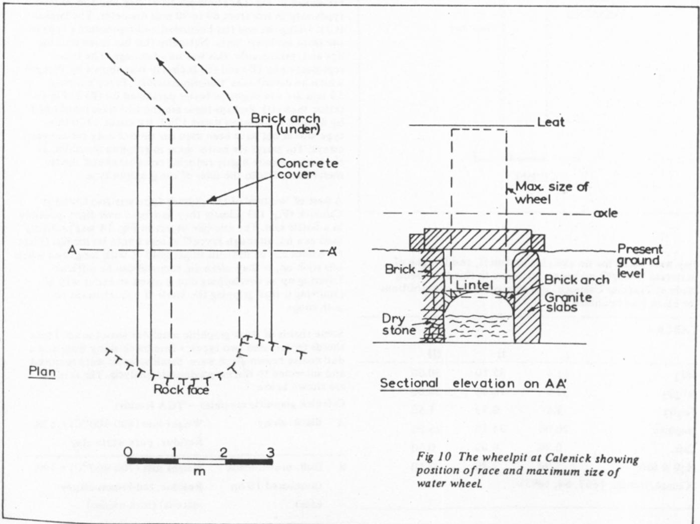
Fig 10 The wheelpit at Calenick showing position of race and maximum size of water wheel.
