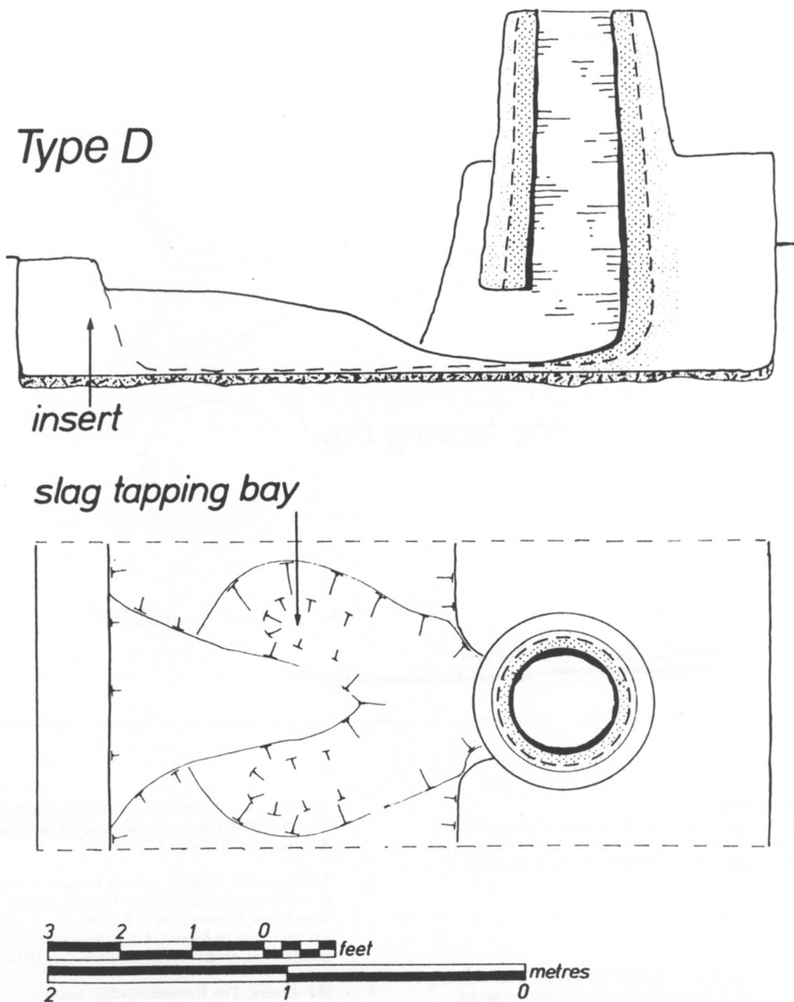
Fig 5 Reconstruction of a single insert
