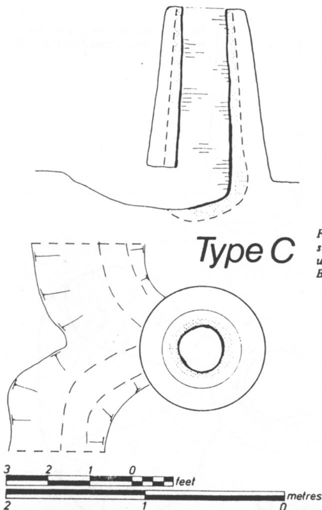
Fig 3 Reconstruction of a free-standing shaft-type smelting furnace using a common slag tapping bay. Broadfield Type C
