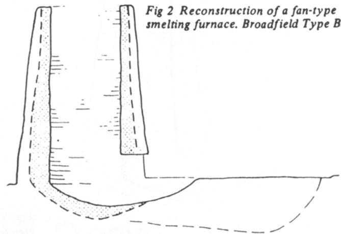
Fig 2 Reconstruction of a fan-type smelting furnace. Broadfield Type B
