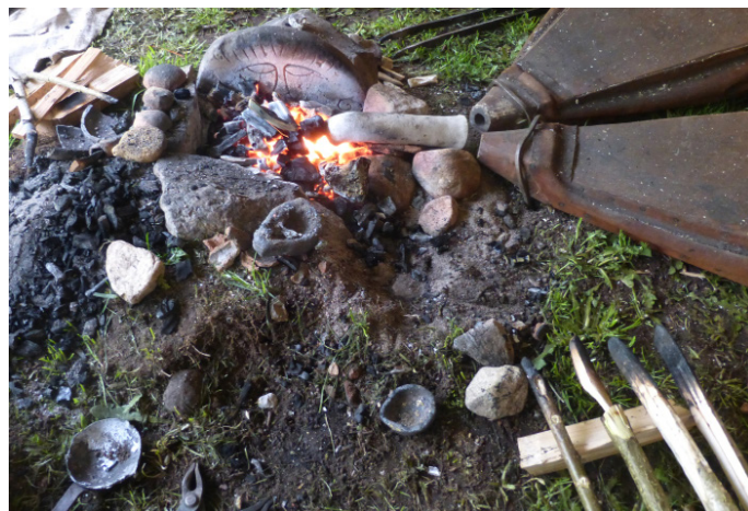
Experimental copper melting and refining using wood and bone rods.
