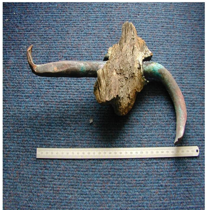
*Fig. 2 Copper bolt from HMS Pomone*
