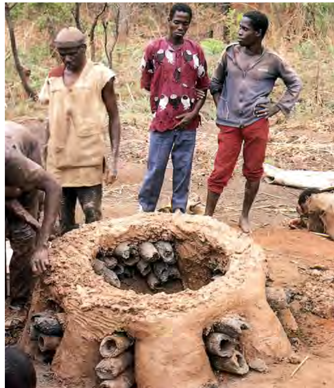
Natural draft low-shaft furnace with numerous tuyères (photo G.Celis).
