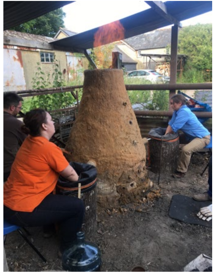
Figure 4: Large bloomery furnace in operation with four drum bellows (Photograph courtesy of C. Livingston).
