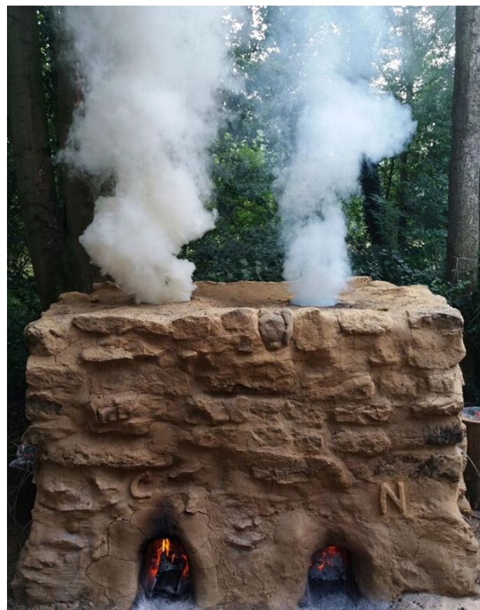
Fig 1: Middle Kingdom smelting furnaces dedicated to wood (left) and charcoal (right) at Aubechies
