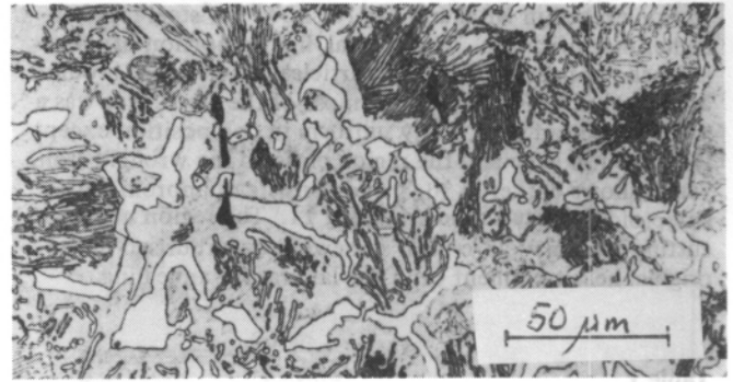
Figure 10. Detail of Figure 9. Structure of light central part of steel layer – annealed
