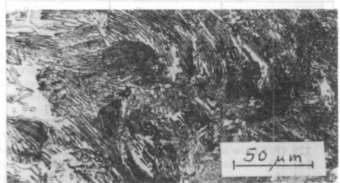
Figure 11. Detail of Figure 9. Structure of dark part of steel layer – annealed
