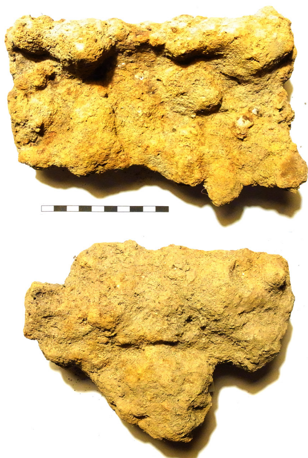
Figure 2: The cast iron pig fragments. Scale 100mm
