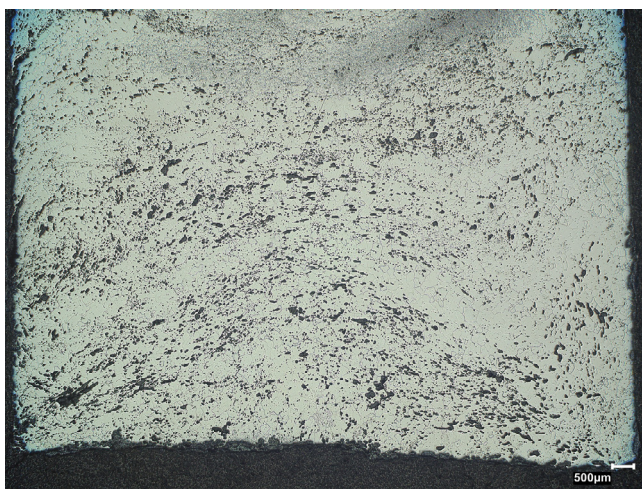
Figure 3 (left). Cross section of a nail from the Weald c.1650. Note the enormous amount of slag and the dark areas of high carbon content.
