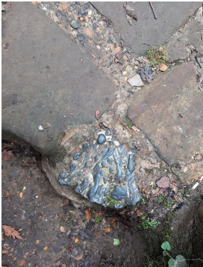
Figure 2. Tap slag, possibly Roman, reused in the later Quarry Garden at Standen. Here it has been incorporated into steps leading into the former quarry.
