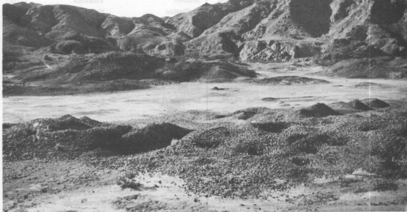
Figure 1 Mining and smelting area of Lasail (Oman). The gossan (centre) was recently levelled. The holes in the slag heap may form by reworking the slag.
