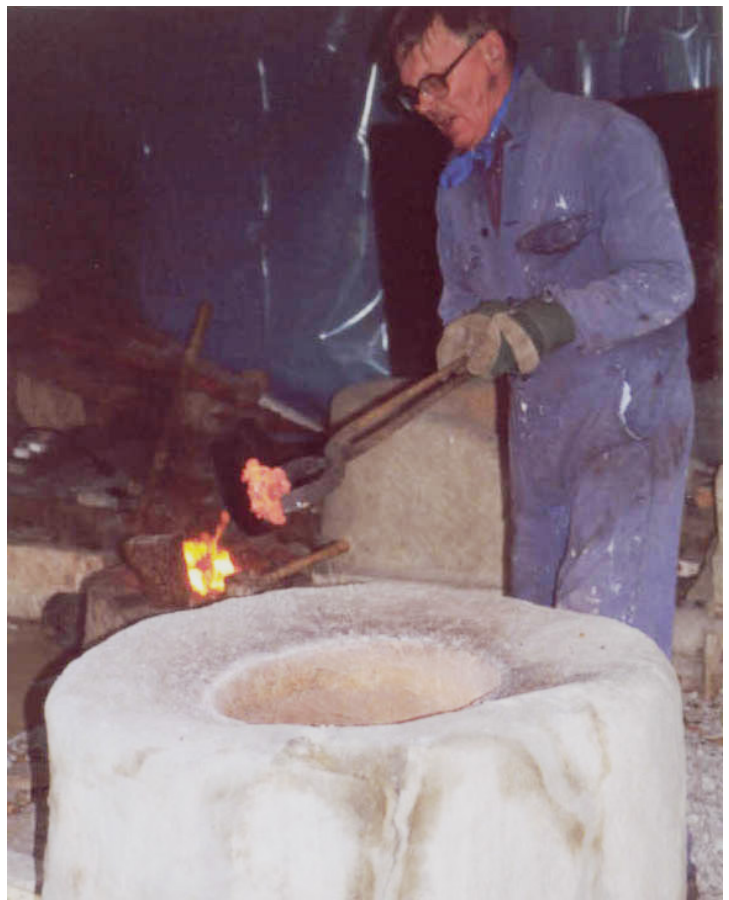
Figure 4: Peter removing a bloom from one of his experimental furnaces
