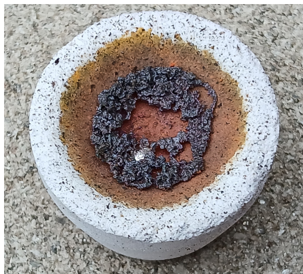
Figure 5: Cooled cupel with slag ring and visible silver bead (photo: M. Straßburger)
