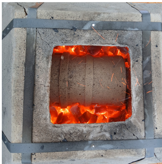
Figure 3: View into the assay furnace during heating (photo: M. Straßburger)
