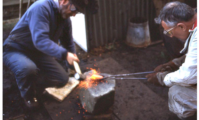
John and Gerry (in white overalls) near the end of welding the pieces of the XP21 billet.
