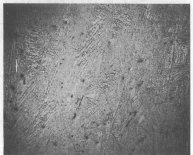
Figure 2. Microstructure of cast irons etched in Stead's reagent. A - grey iron, at x 1.5; B - mottled iron, at x 8; C - white iron, at x 8.
