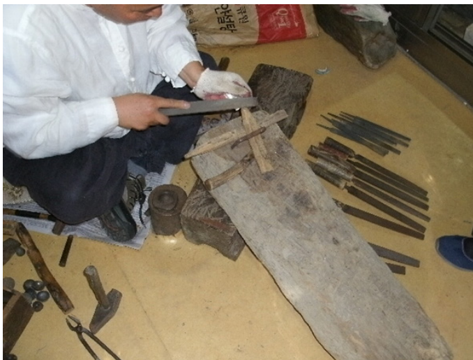
Figure 6. The plate is filed to remove the low melting silver alloy from the surface leaving it only in the chased designs
