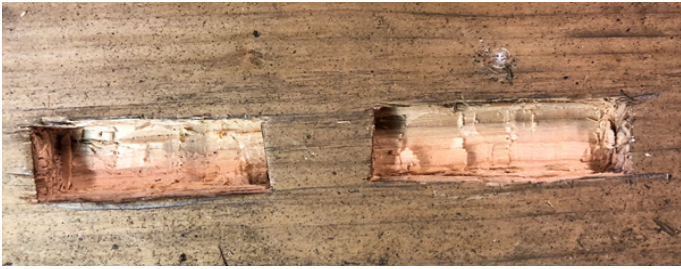
Figure 2 Notches cut into a pine wood board with a chisel approximately 2" x 1/2" x 3/8" deep
