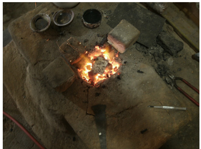
Figure 5. The square light coloured plate in the centre of the charcoal hearth is carefully heated and the special silver alloy melted over it
