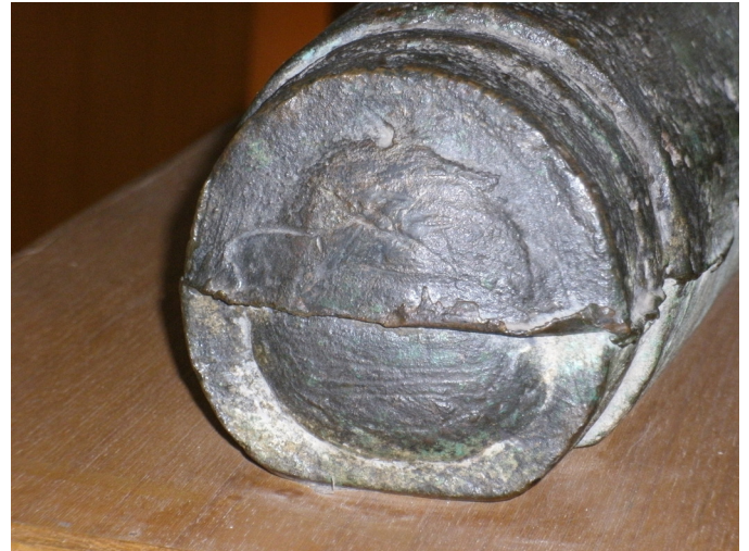
Fig. 2 Mouth of the cannon. Note the feeding head, or sprue which would have been sawn off before drilling commenced, and the prominent flash lines (P. Craddock).
