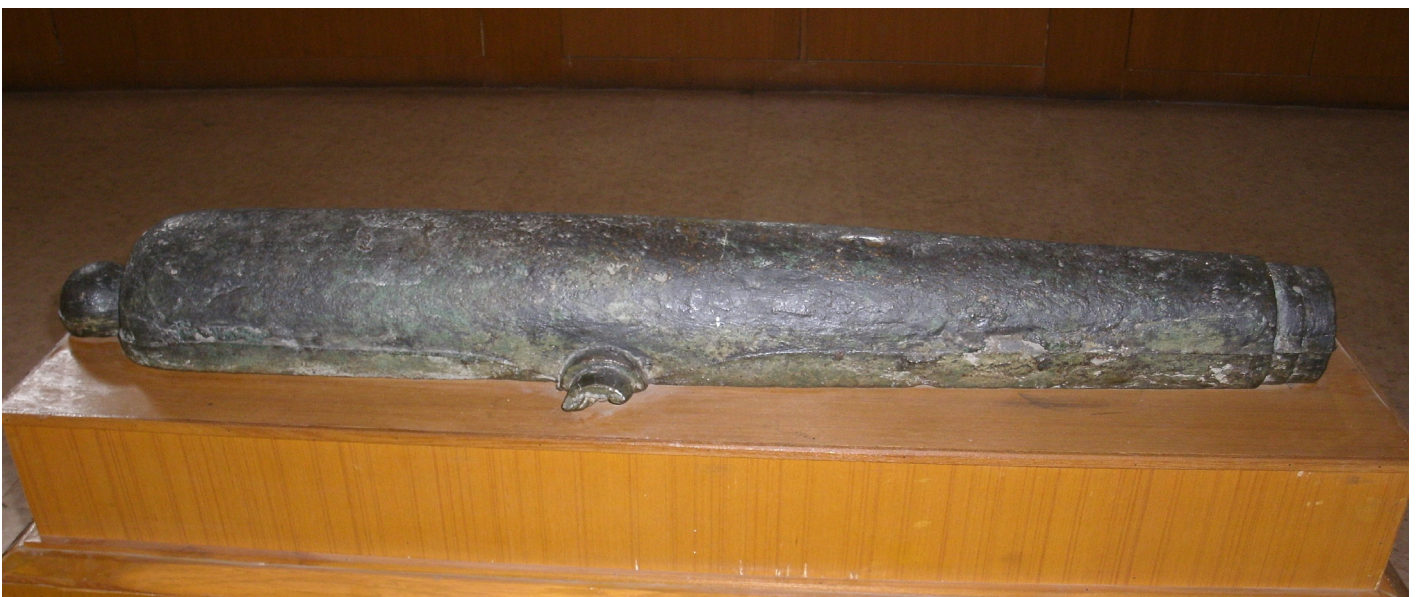
Fig. 1 Small copper alloy cannon barrel now in the Indore museum. The casting was misaligned in the mould and abandoned. Note the flash lines running continuously all around, showing this was cast in a two piece mould (P. Craddock).
