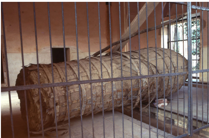
Fig. 3 Complete, unused mould for casting cannon, probably 18th -19th century, at the Jaigarh Fort cannon casting foundry. Note the iron binding bands (P. Craddock 2015).
