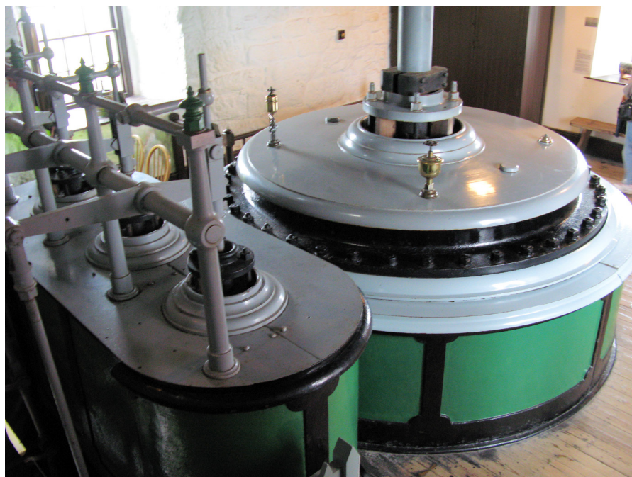
Figure 3 (below): The 90" steam cylinder and valve bank of the East Pool steam engine.
