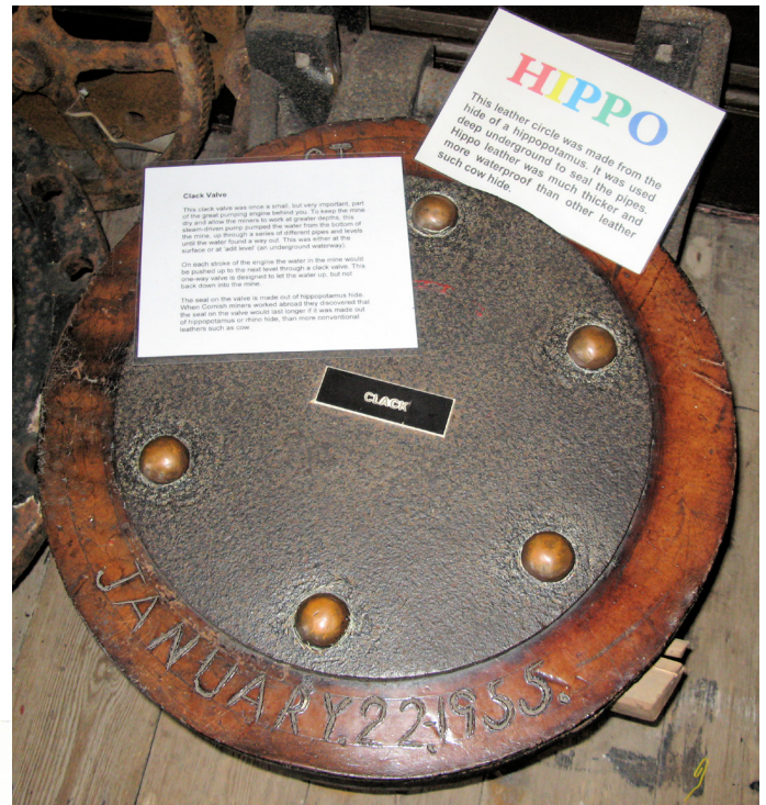
Figure 2: Clack valve made of Hippopotamus hide, a superior material to cow leather.
