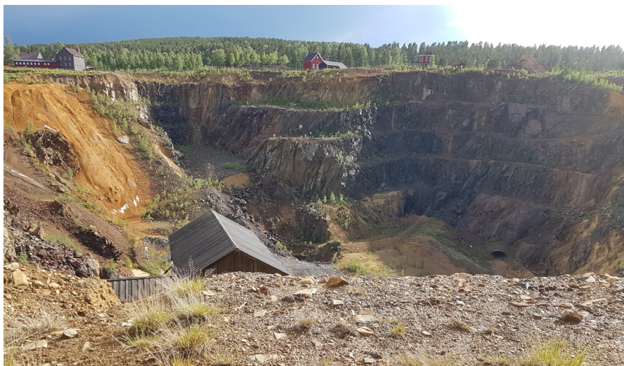
Figure 3 (left): The Falun mine's maze of galleries collapsed in 1687 leaving this pit, over 90m deep.
