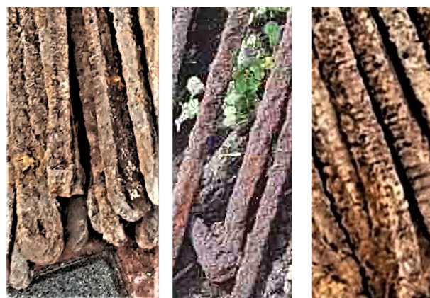
Figure 3: 1: Folded bars. 2: hook on bar No 2; 3: notches on the face of bars.
