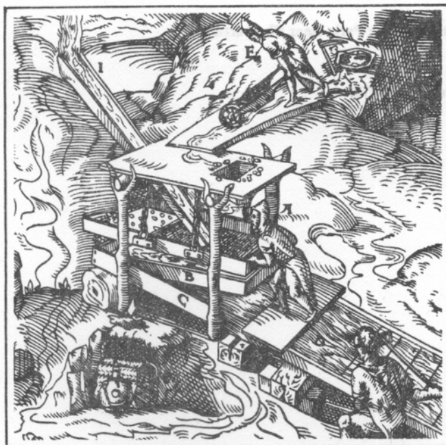
Washing alluvial gold ores. Lazarus Erker, UCP translation p 99.
