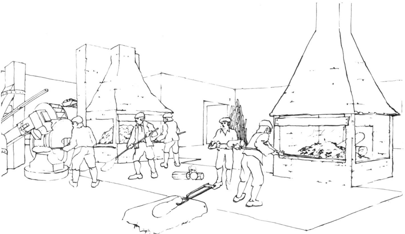
Fig. 1 — The interior of a Walloon forge at Forsmark, 1793 (after Hillestrom)
