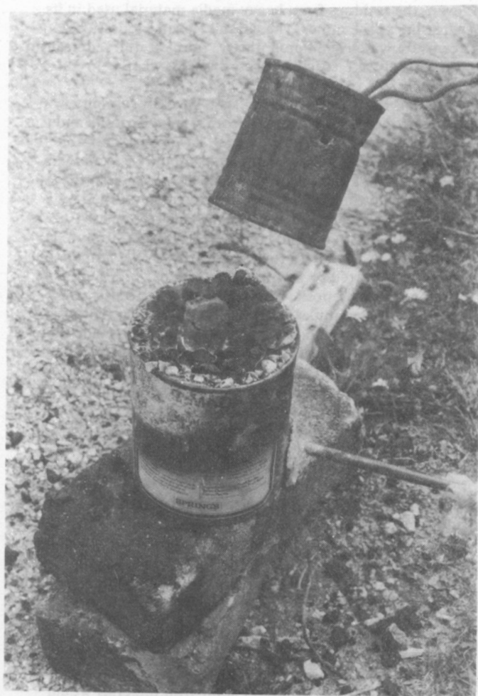
Fig 4 Fire assay. The crucible holding the sample-charcoal mix in the furnace at the start of the heating. More fuel is about to be piled over the crucible and the furnace cover put on. The temperature will be raised to 'bright yellow' by blowing. Dia of containers = 10 cm. Dimensions of crucible for the small fire assay used in the work: 3 cm od x 4.5 cm high; wall thickness 3 to 5 mm, hemispherical base.
