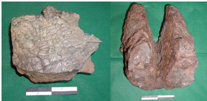
Figure 4 (left). Ripples on a piece of slag, which had solidified against the cold wall of the slag pit. Each ripple may represent decantation of some 10 kg of slag. From Vårhussetra. Figure 5 (right). Typical primary bloom, obviously taken hot out of the furnace and immediately split with an axe. Weight 17 kg, slag free, low in phosphorus and with 0.26 % carbon. Density about 6, due to large cavities. In the possession of the museum in Trondheim. Photographs by AE.
