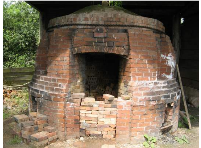
A working reconstruction of a small Victorian beehive-type brick kiln, photographed at the Acton Scott Museum, Shropshire. A kiln of this type and size may have fitted quite comfortably within the redundant cone/hovel of Bedlam’s “Furnace II”.
