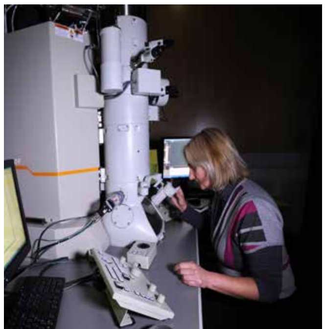
At work in front of our Jeol 2100 TEM with Vulcan Cathodoluminescence detector and EELS spectroscopy
