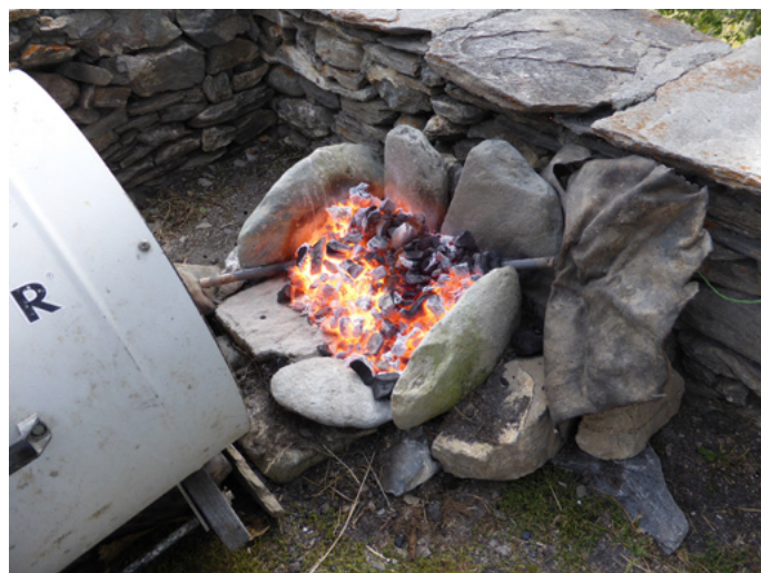
Figure 4b Reconstruction of an Ujina-Collahuasi bench-shape furnace for a smelting experiment; a 40 km/h -1 wind was produced with an industrial fan.
