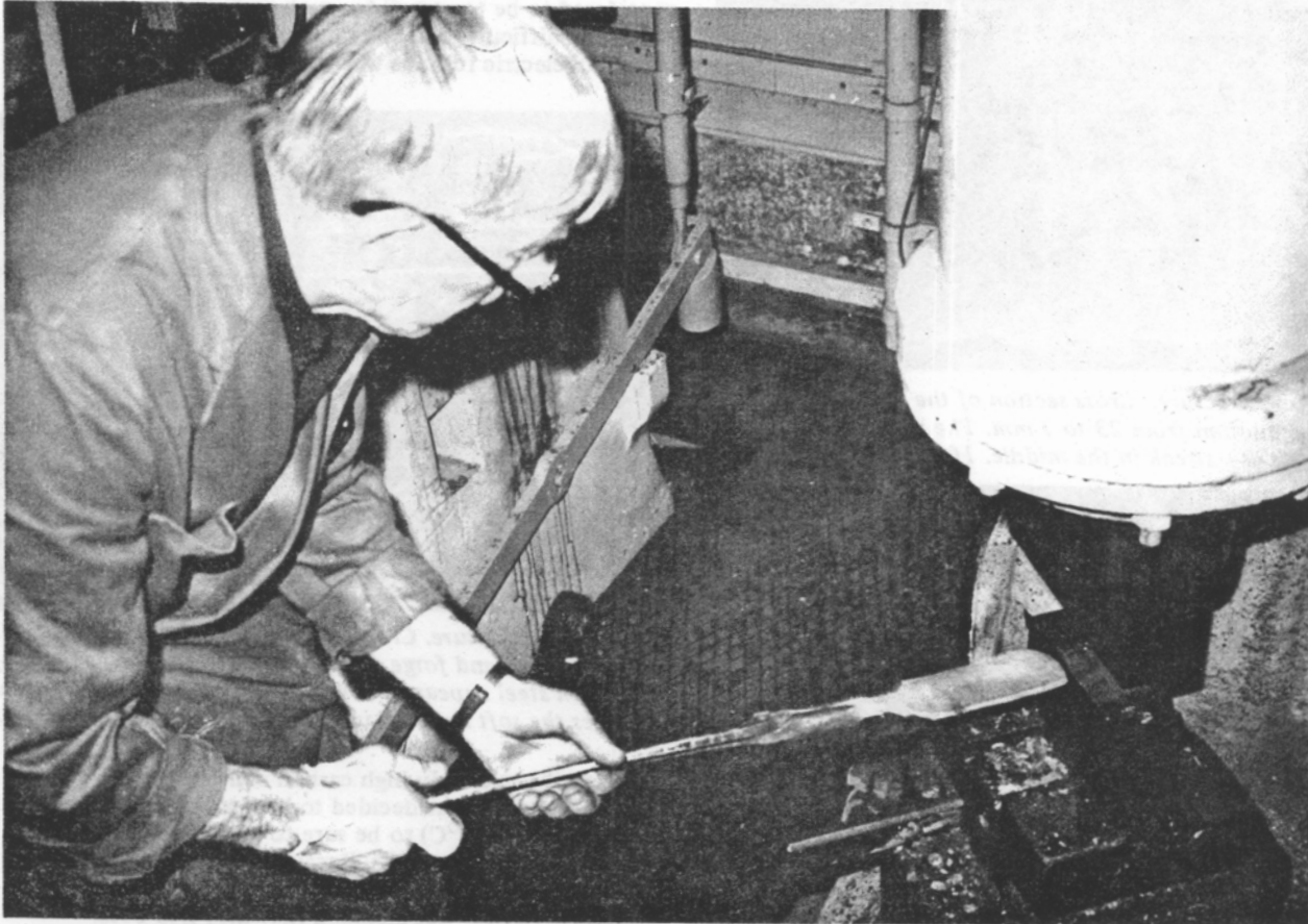
Fig. 2 The forging operations were made under a pneumatic hammer.
