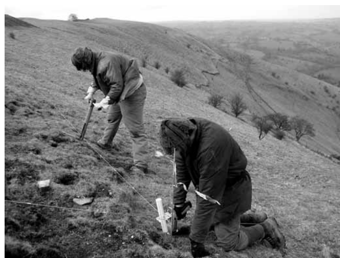
Figure 1. Geochemical prospection at Ecton Hill using portable XRF (note mining spoil and Bronze Age barrow in background)
