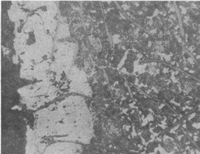
Fig 9 Laboratory-produced coating of the Cu-Sn-Pb alloy on the cut surface of a piece of grey iron. Note how the liquid copper alloy has dissolved the metal matrix of the cast iron without disturbing the graphite flakes which lie both in the coating and the cast iron. Magnification: x200.
