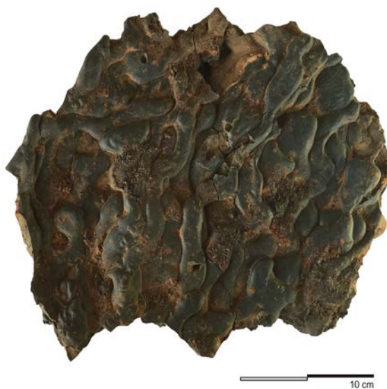
Fig. 5. Typical tap slag cake from A Veiga de Escouredo showing ropey flows on the upper surface
