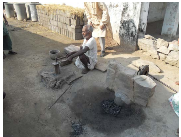
Fig. 9. Smithing workshop in the village of Nagaram, Telangana, South India (Pioneering Metallurgy Project 2010). Note the stone built charcoal-retaining wall of the hearth.
