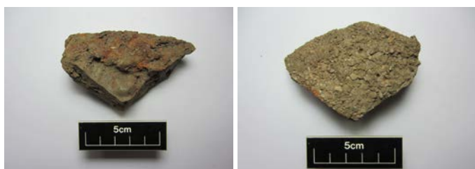
Fig. 5. Example of smithing hearth slag cake with sand on the underside
