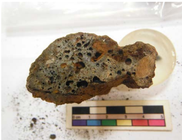
Fig. 3. Cut section of a lump of slag recovered from As Mestas , showing large inclusions and corrosion by-products
