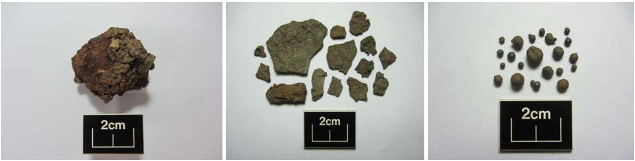
Fig. 8. Small iron bloom fragment (left), hammerscale flats (centre) and spheroidal hammerscale (right)
