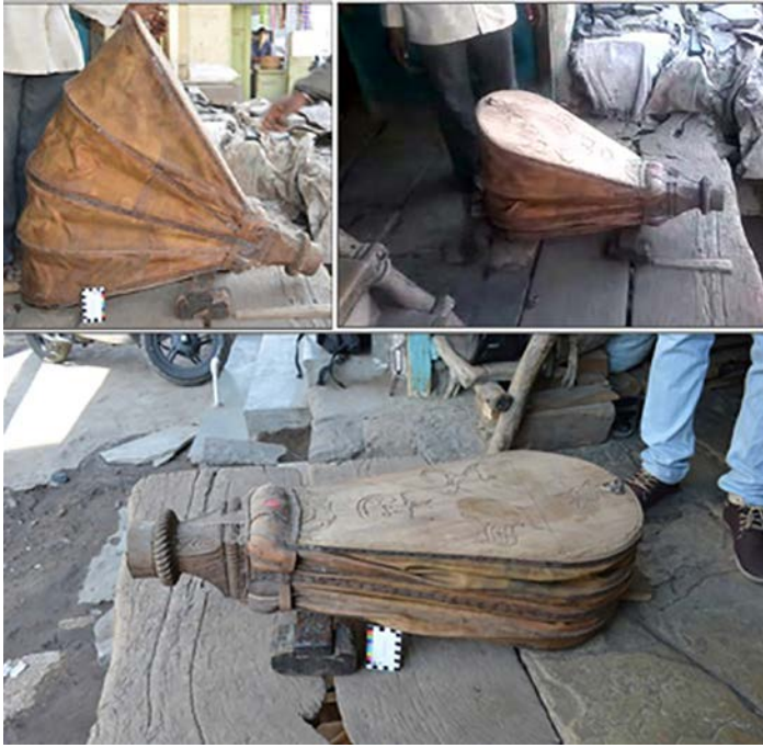
Fig. 3. Bellows made in the Sholapur workshop
