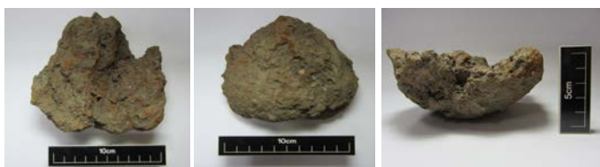
Fig. 4. Example of a smithing hearth slag cake from Blihun Hanben
