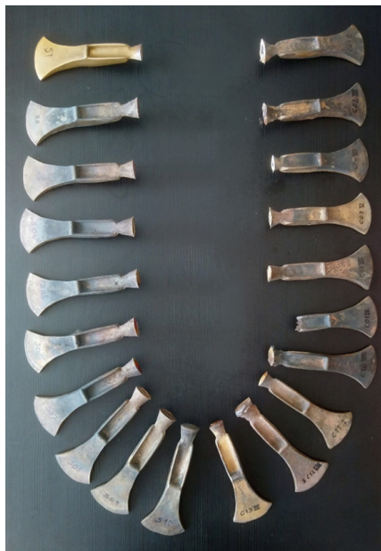
Figure 1 (left): To the left: Ten palstaves cast in the soapstone mould. To the right: Ten palstaves cast in the clay moulds. Note that one is only partially cast and that the sprues are still attached, and that flashing has been removed
