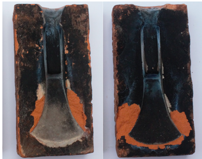
Figure 4: Typical damage to the clay moulds after (Left: One valve from CI. Right: One valve from CVII)
