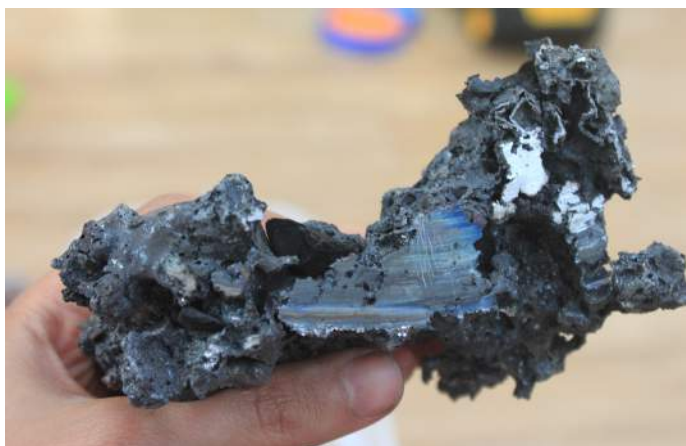
Cross-section of the bloom produced from Furnace 1.
