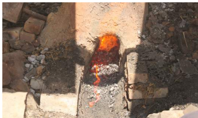
A trickle of slag during the tapping of smaller furnace 1. ores were placed to the side so we could conduct our first experiment using a local hematite (pre roasted and beneficiated by Jake) in the smaller furnace.
