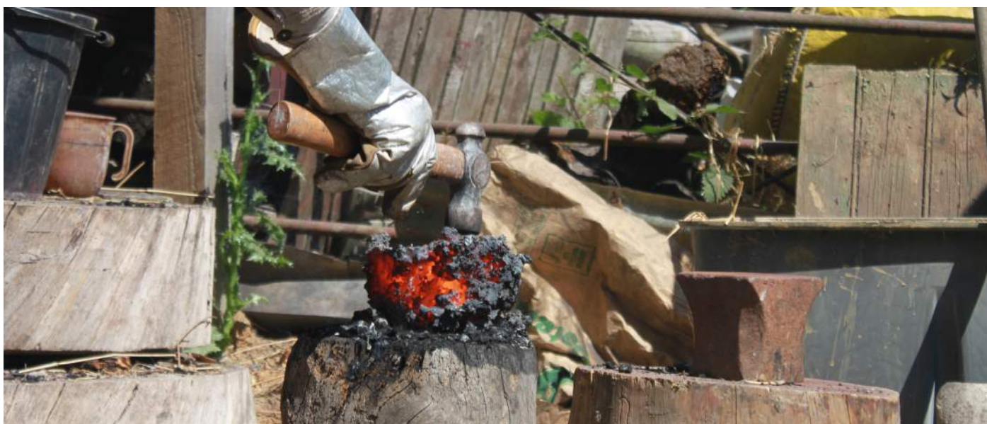
A bloom just been extracted from the smelting furnace consolidated by hammering.
