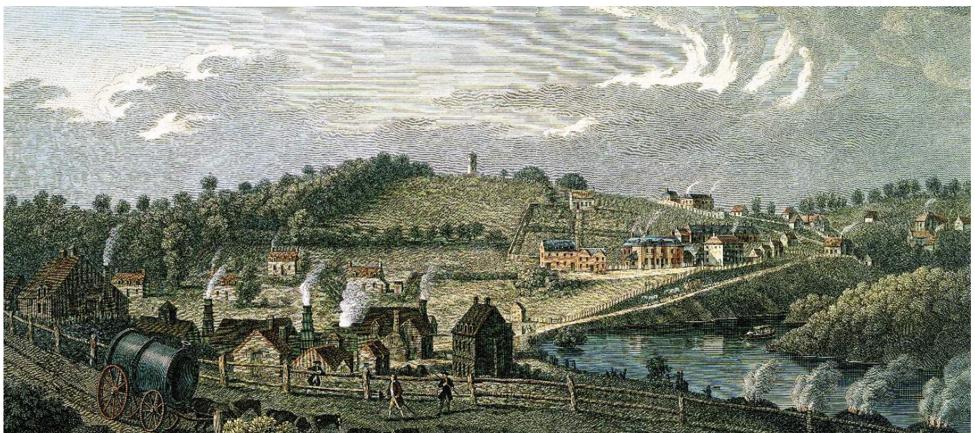
The Coalbrookdale of Abraham Darby II- 'View of the Upper Works at Coalbrookdale' 1758 by Francois Vivares. Note the cast iron steam engine cylinder in the foreground. © Ironbridge Gorge Museum Trust
