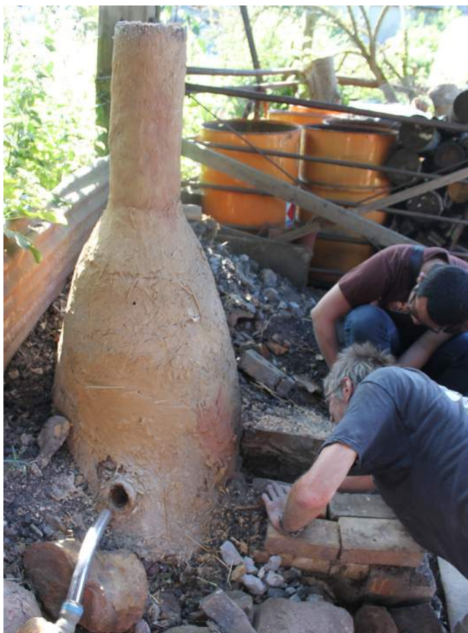
The smaller furnace 1 operated with vacuum cleaner bellow
