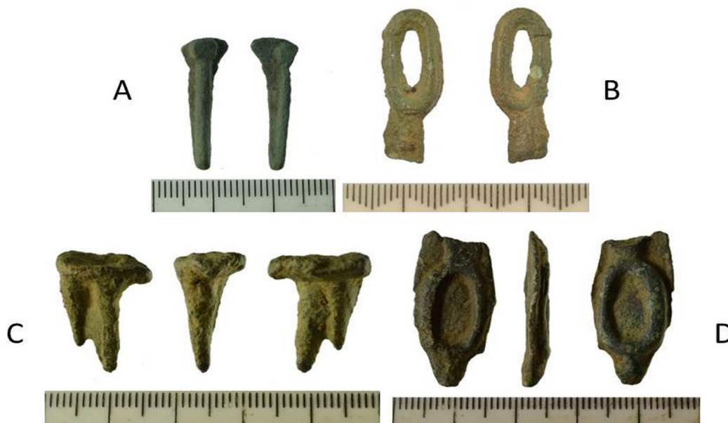
Fig. 1. A badly cast pin, misaligned as well as flashing; B: Failed cast of another buckle; C: Double sprue with flashing; D: Failed cast of a buckle
