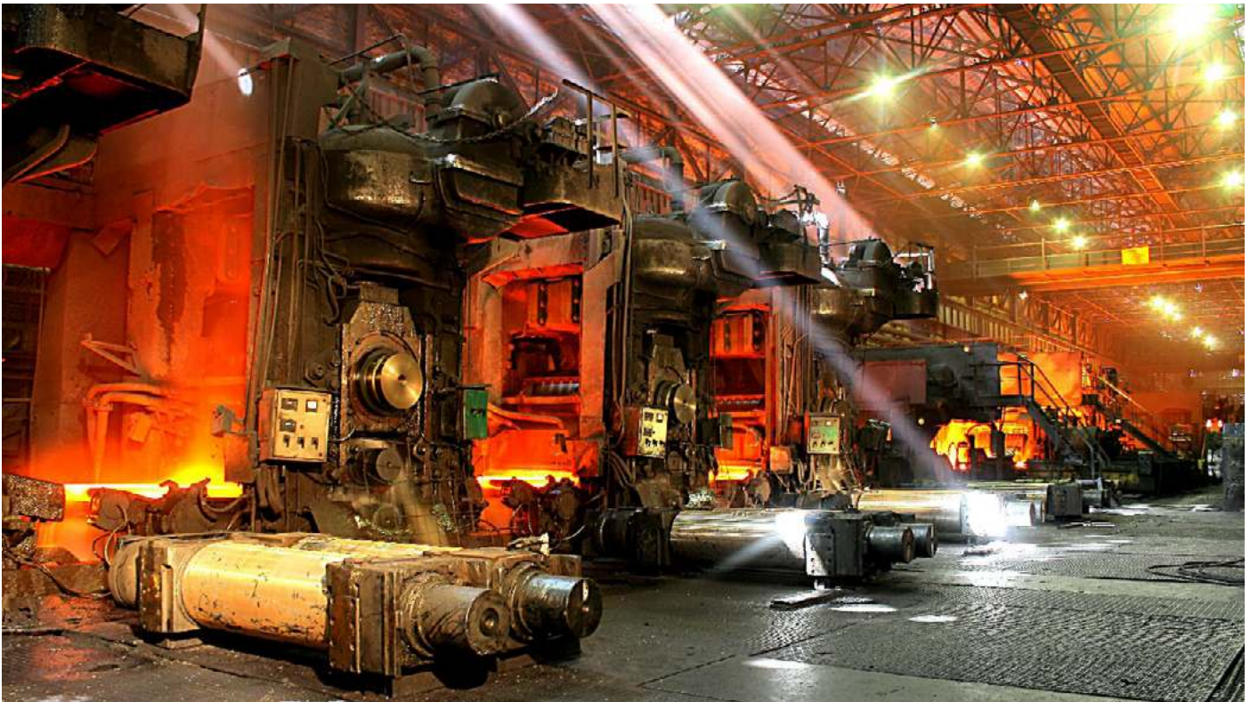
The wide hot strip mill at Zaporozhy, Ukraine was supplied by United Engineering of Pittsburgh in 1938 and is still in operation today making it Europe's oldest continuous hot strip mill.
