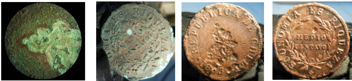
Fig. 5 The before (5 a. and 5 b.) and after (5 c. and 5 d.) of the 1853 historical copper coin to electrolytic cleaning and macroscopic images.
