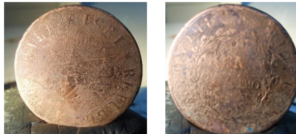
Fig. 6 Inverse and reverse of 1851 historical copper coin after the electrolytic cleaning.
