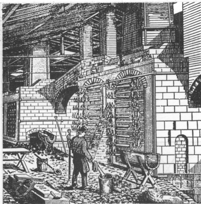
Figure 5 Inside a nineteenth-century Belgian zinc works, showing distillation furnaces, with condensers protruding. (From W C Roberts-Austen: Introduction to metallurgy London: Griffin, 1902)
