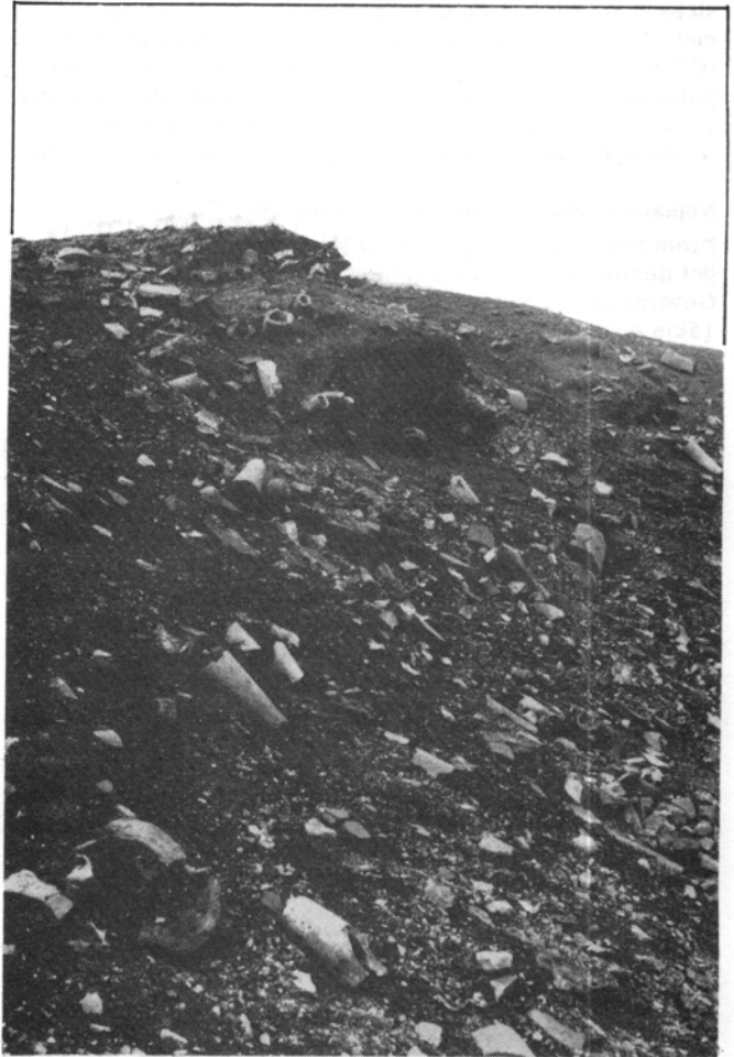
Figure 8 Zinc-smelting residues remaining on a part of the Tindale site, 1975. Fragments of conical condensing tubes can be easily distinguished, together with pieces of the larger fireclay retorts.
