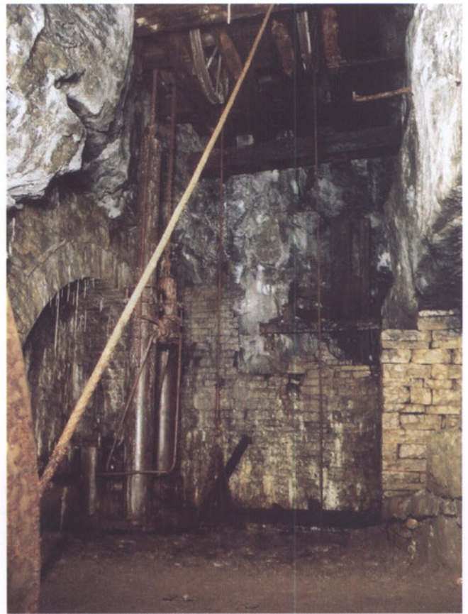
Figure 9: The sub-surface of a lead-mining landscape at Gunnerside Gill, North Yorkshire. This engine house is on Sir Francis Level 240ft below the valley (Fig 35). Two Davey hydraulic engines were installed in 1880: one (centre left) worked the pumps (two large vertical pipes) and another (behind camera viewpoint) the winding gear. One cage is suspended just below floor level.
