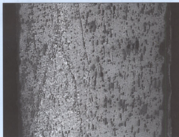
Figure 22: Section through knife blade. The varied texture to the left shows the incorporation of several pieces of scrap metal. Image width ~1.5mm.
