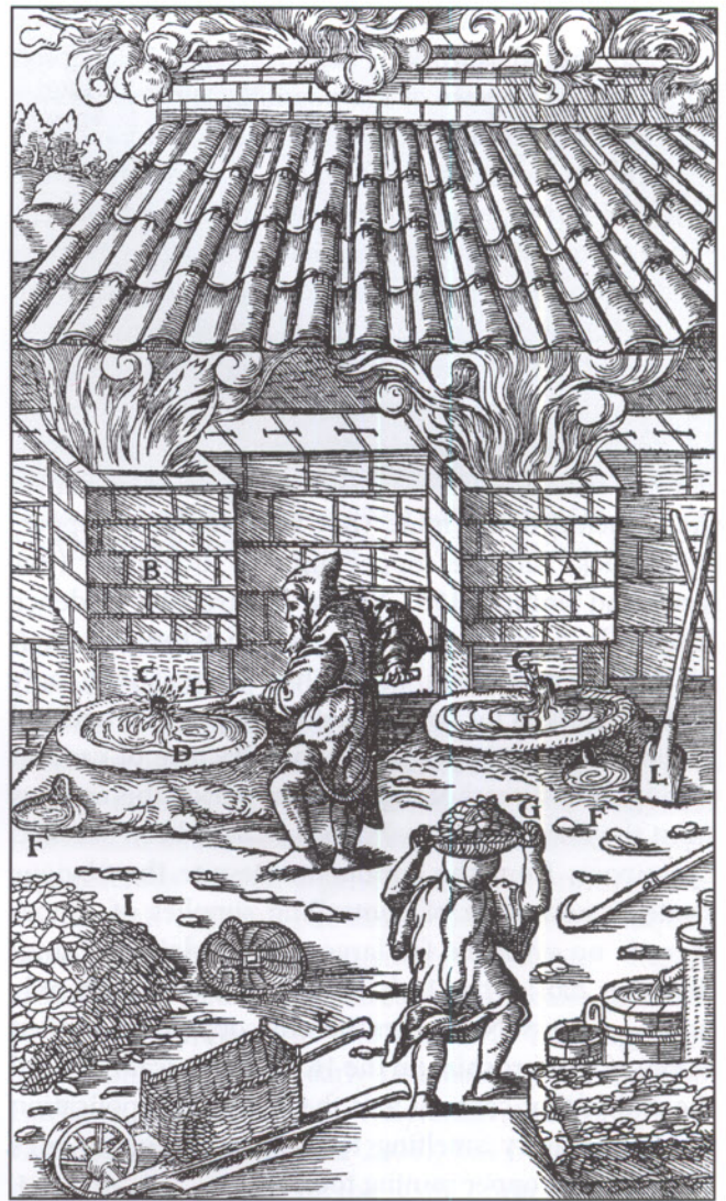
Figure 68: Agricola's illustration of 16th-century copper smelting in Germany. After Hoover and Hoover 1950.
