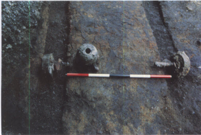
Figure 81: Early-18th-century gun-boring mill at Pippingford, East Sussex. Two of four trolley wheels are shown, with rotted timber rails. The hemispherical object is a chuck to hold a boring-bar, as seen in Fig 80.
