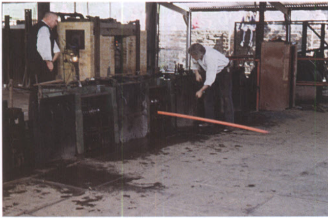
Figure 30: Red-hot wrought iron being rolled at the re-erected rolling mill at Blists Hill, Ironbridge. Traditional metal-working skills are being preserved as 'living history'.
