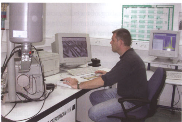
Figure 46: Scanning electron microscope in use. The main screen shows an image of the sample in the chamber to the left, at high magnification, while the screen to the right displays the results of EDS analysis.
