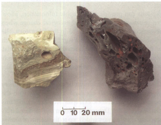
Figure 17: Blast-furnace slags are usually glassy in appearance and can range in colour from blue/green through to grey/brown. They were often re-used as hardcore and so can be found in small pieces far away from furnace sites.
