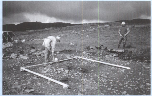
Figure 31: Magnetometer survey at Geli Goch, Gwynedd using a 4m-square frame at a sensor height of 320mm. To the right of the furnace is the working pit, with the last run of tap slag still in situ.
