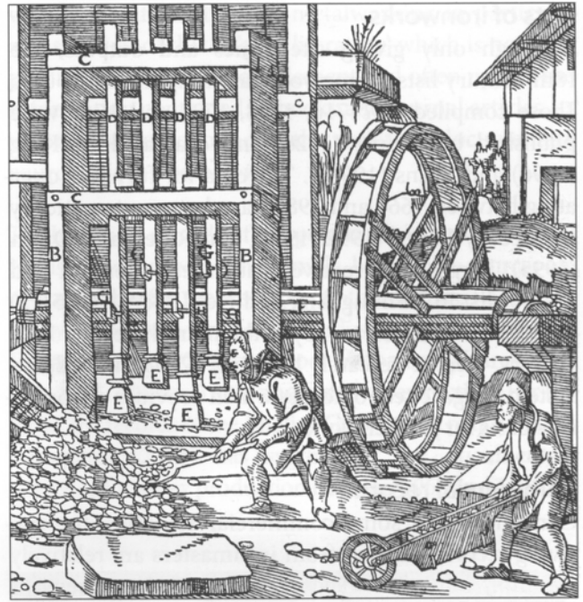
Figure 24: Water-powered stamp mill crushing ore in Germany in the 16th century from Agricola's De Re Metallica . After Hoover and Hoover 1950.
