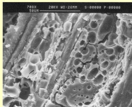
Fig 5.2.4 (below right) An SEM image of wood showing that the structure appears to be filled with resin or wax.
