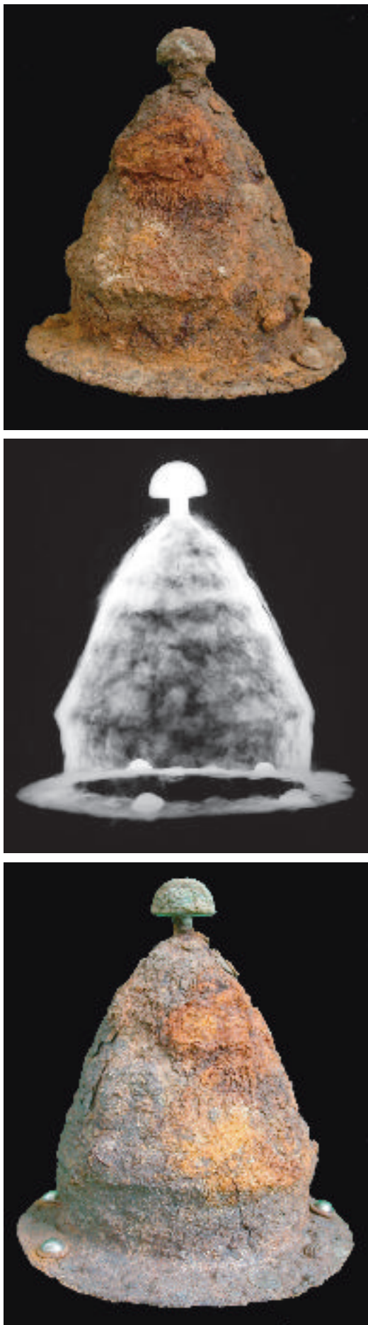
Fig 16 Early medieval shield boss as excavated (upper). The X-radiograph reveals hammer marks aligned around the apex from forging the iron boss to shape (middle). The studs are made from silver alloy and thus show in the radiograph due to differences in metal composition. These were revealed during conservation (lower).
