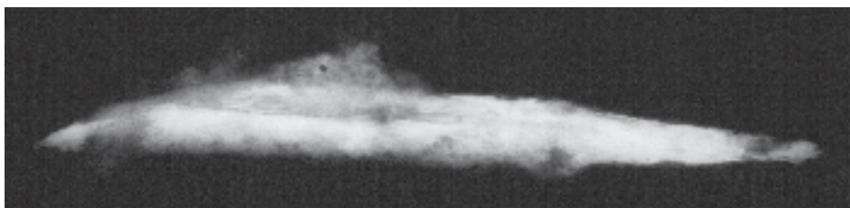
Fig 11 (below) Early medieval knife with pattern-welding in the back of the blade. Length: 178mm. Exposure: 3mA, 110kV, 60s, 0.45m FFD, Kodak Industrex MX.
